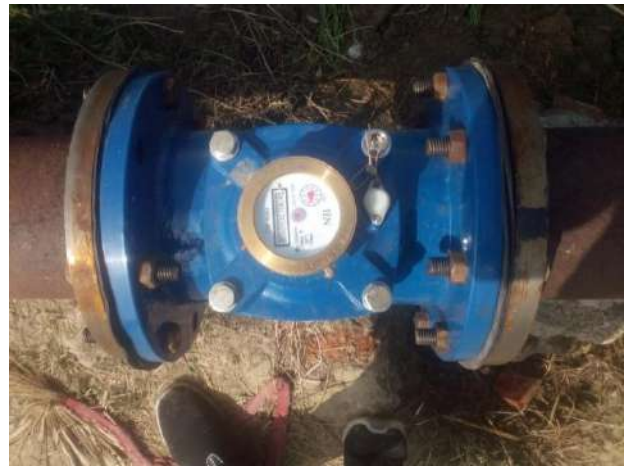
Fig. 8.2. Pictorial view of setting water flow meter for discharge measurement
