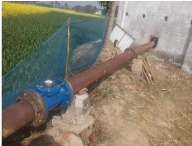
Fig. 8.2. Pictorial view of setting water flow meter for discharge measurement
